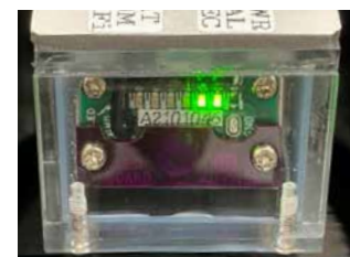
When the main power is switched on, 2 LEDs will light up
