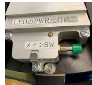
Main power switch (on inside of wheel)
