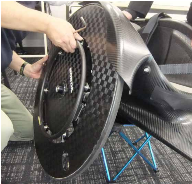
Attach the wheels to the wheelchair frame
