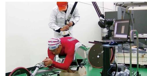
Analysis of cornering forces on frame structure
